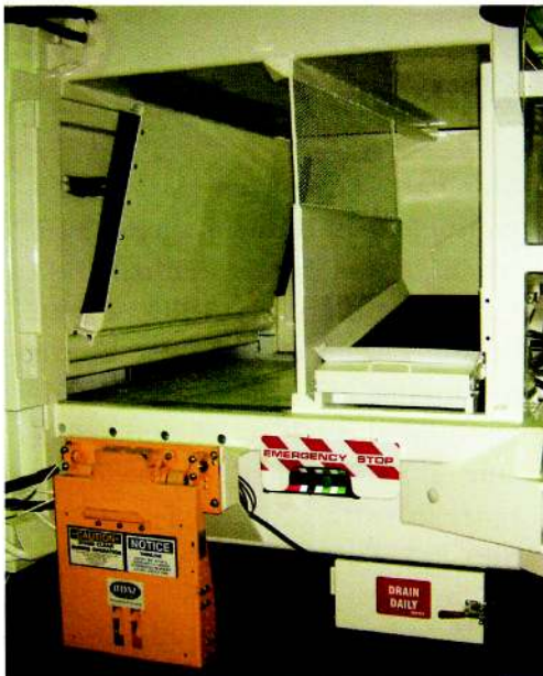
FEEDING THE NEED: A hydraulic conveyor feeds waste deep into the truck. (Photo: Shu-Pac)
