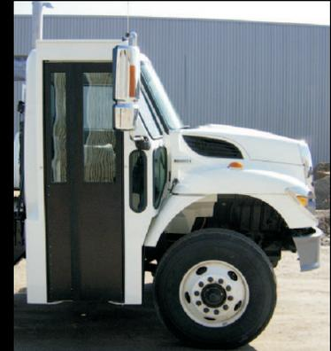
≡ Automated bifold doors open with work-brake and close when operator returns to cab.
