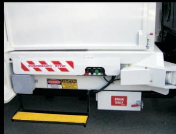
≡ Hopper steps with integrated safety pads to interrupt power.
